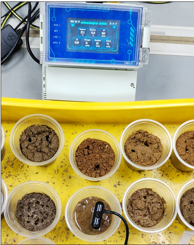
Figure 3. Soil parameters determination using EC-based electronic nutrient sensor (Shandong Jingxunchangtong Electronic Technology Co., Ltd., China)
